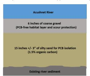
Example Cross Section of Typical Cover/Cap
