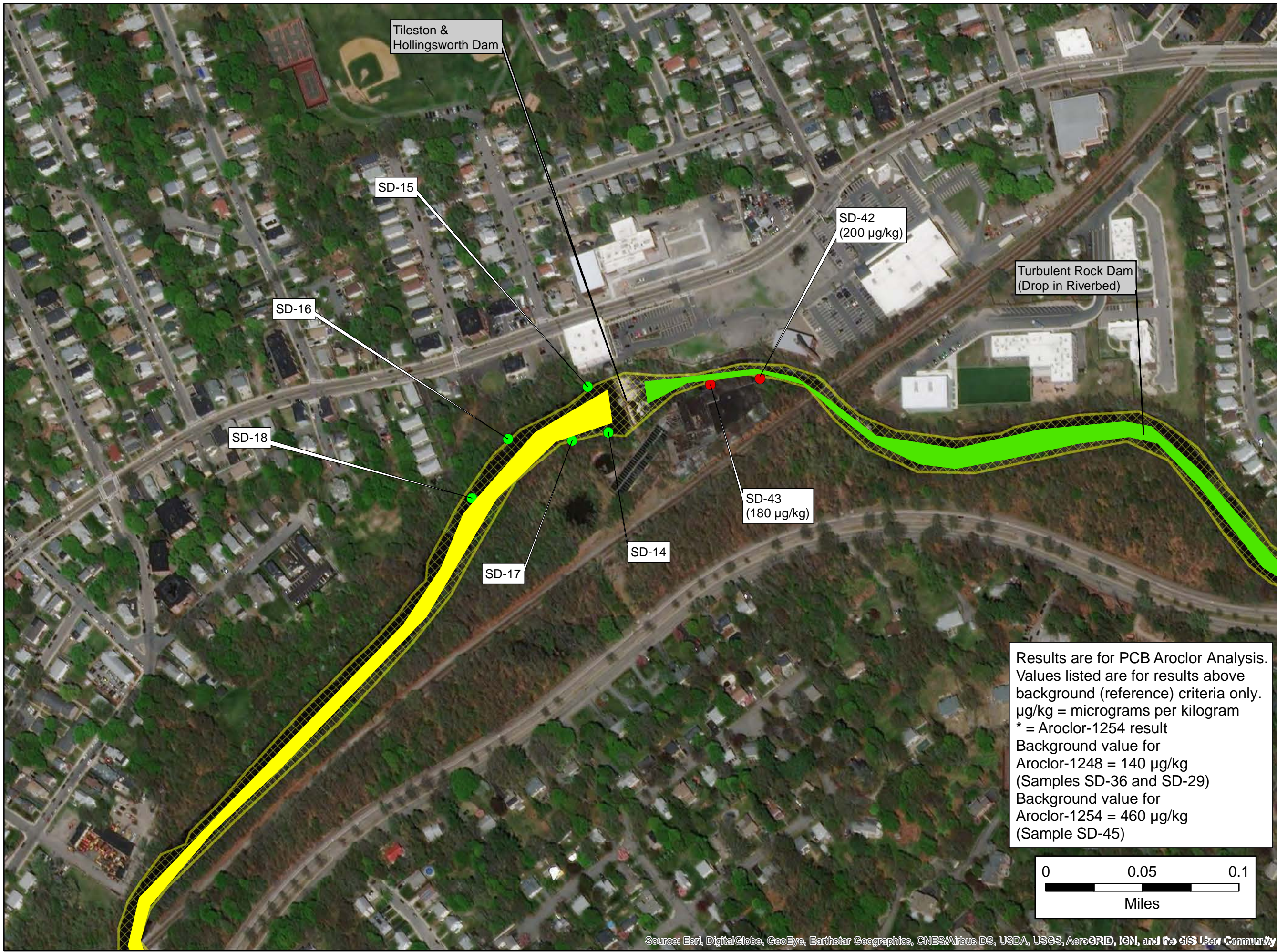
Figure 7D 2017 START Sediment Sample Locations and Results Map (Tileston & Hollingsworth Dam and Blue Hill Ave Area) Lower Neponset River PCBs Boston/Milton, Massachusetts
