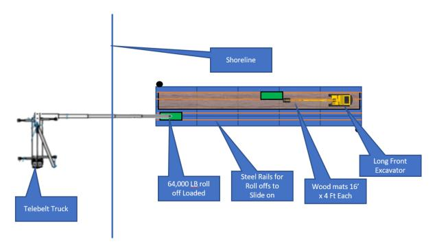
3) **<u>Comment</u>**: Are any tracking problems of the roll-off boxes anticipated across the travel path on the barges, that may necessitate rails of some sort?
