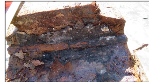
Figure 14. A flat-nibbed scarf joint (left-side images) was used to connect NBHSS UAD SW#2's fore and aft keel sections. The joint was fitted with two stop-waters (right-side images) to prevent water from traveling along the seam into the hull (photographs by David S. Robinson, DSRA).
