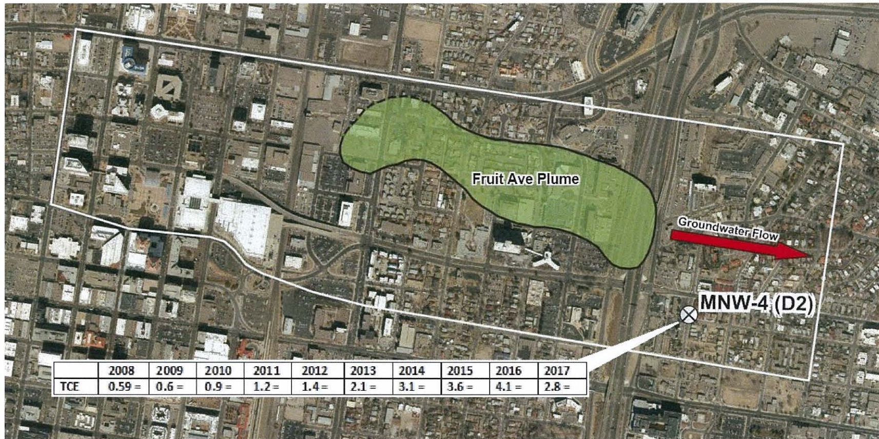
Figure 1: Map of trichloroethene (TCE) plume at aquifer depth interval 2 (D2; 4,752 to 4,647 feet above mean sea level) with defined (solid line) and inferred (dashed line) plume boundary showing concentrations of TCE greater than 5 micrograms per liter in February 2017. Table summarizes the detected concentrations (=) in micrograms per liter of TCE found at monitoring well 4 (MNW-4 (D2)) from 2008 to 2017. Map created by Kate Mendoza, August 2017.
