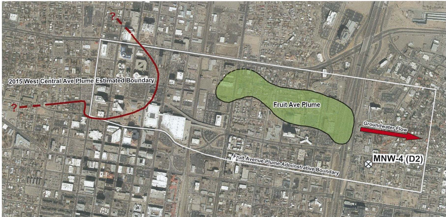
Figure 2: Map of the West Central Avenue trichloroethene (TCE) plume encroaching on Fruit Avenue Plume Superfund site. Defined (solid line) and inferred (dashed line) plume boundary showing concentration of TCE greater than 5 micrograms per liter in 2015. Map created by Kate Mendoza, August 2017.
