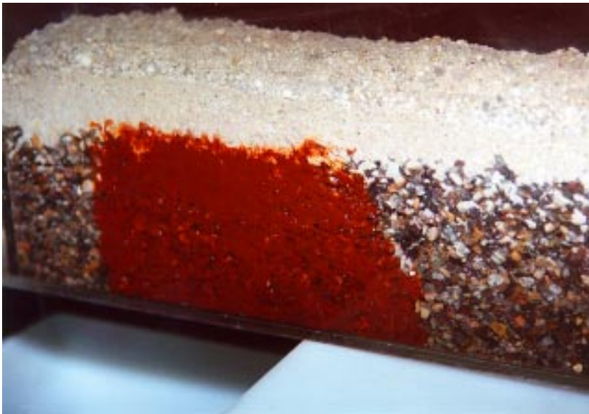
Figure 2.17. Testing hydraulic conductivity of amorphous ferric oxyhydroxide/gravel mixture.
