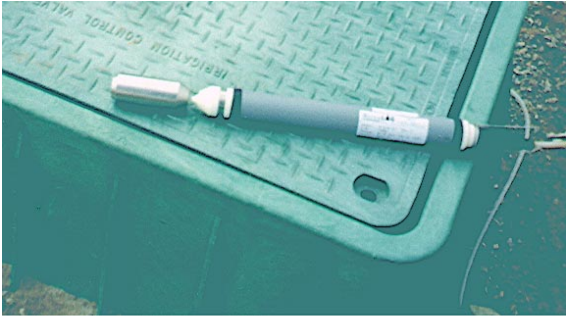
Figure 4.5. Pressure transducer deployed during PRB demonstration, Fry Canyon, Utah.
