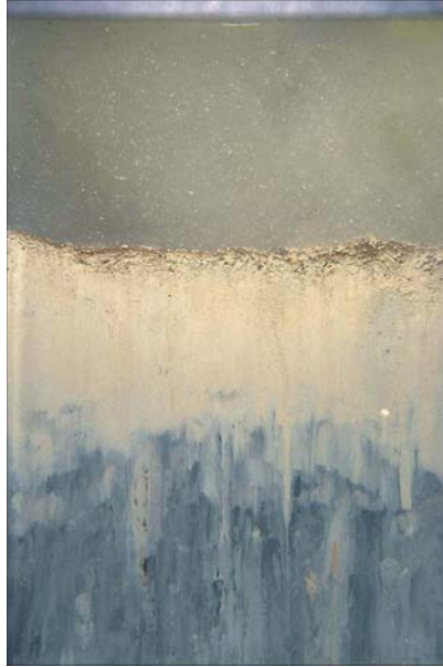
Figure 12. Example of a SPI camera image showing homogeneous clayey silt and RPD (image width, 14 cm).
