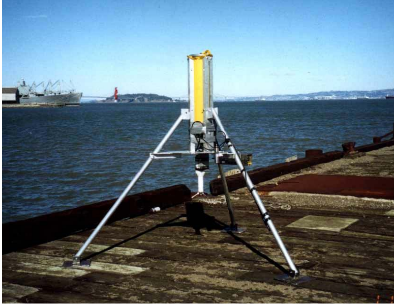
Figure 13. Tripod deployed at HPS to measure hydrodynamic parameters.
