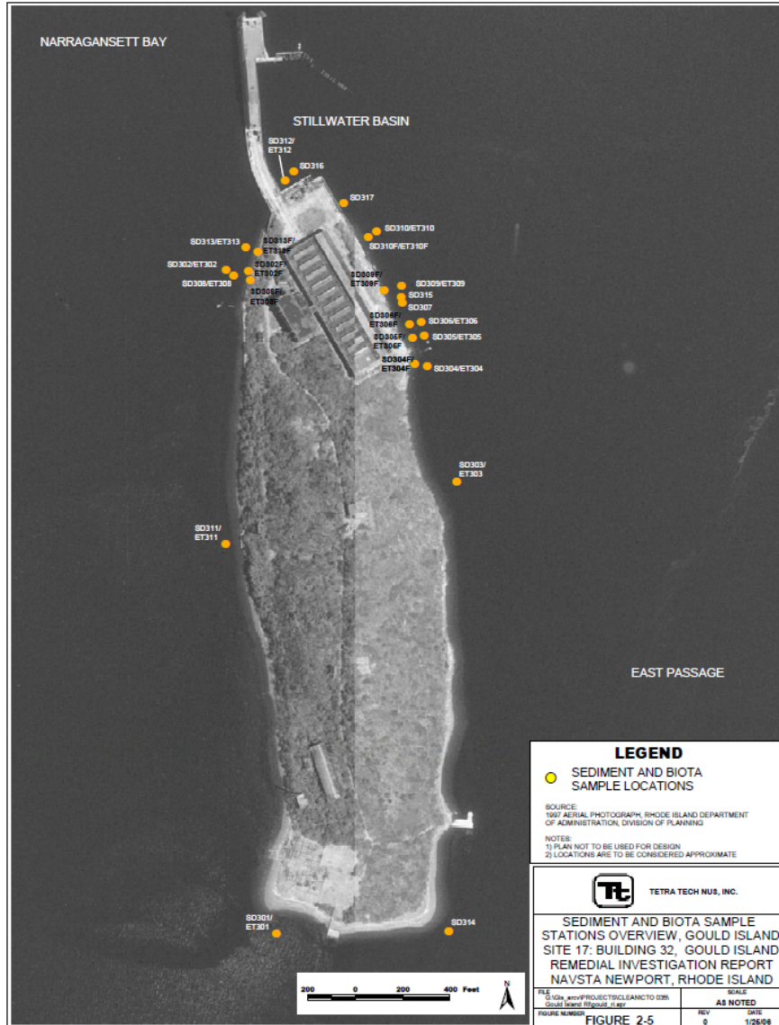
Figure D-2. Site map of Gould Island showing the location of the RI sediment samples.
