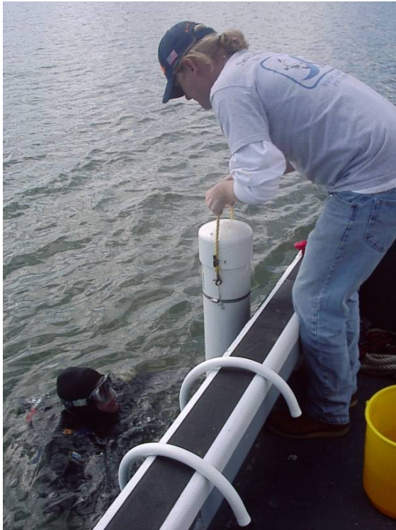
Figure 15. Diver-deployed sediment trap. Photo on right is looking down into a sediment trap, where the brine layer, colored by Rhodamine dye, can clearly be seen.
