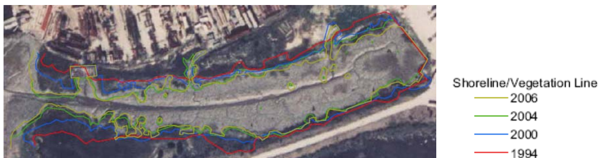
FIGURE A-13. Aerial photograph attests to the continual encroachment of shoreline vegetation into the Barge Canal from 1994–2006. The encroachment of vegetation qualitatively suggests significant sedimentation in these areas.
