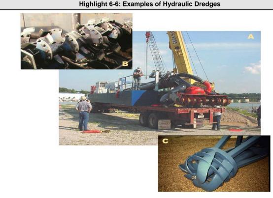
Note: A = Fox River, WI; horizontal auger hydraulic dredge deployment (Source: Jim Hahnenberg U.S. EPA)
