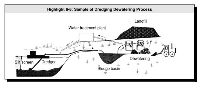
Depending upon the quality of the water after it is separated from sediment and upon applicable or relevant and appropriate requirements (ARARs), it may be necessary to treat water prior to discharge. Where water treatment is required, it can be a costly segment of the dredging project and should be included in cost estimates for the alternative. Water treatment costs may also affect choices regarding dredging operation and equipment selection, as both can affect the amount of water entrained.
