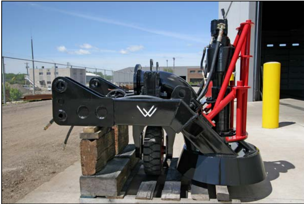
Figure 14. Vic Vac® hydraulic dredgehead for residuals.
