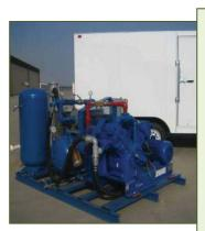
Since 2009, a cryogenic compression and condensation process has been used to recover hydrocarbons from SVE operations at the State Road 114 Superfund site in Levelland, Texas. Over the first seven months of operation, the process brought in project revenue of approximately \$45,000, approximately 70% of the SVE system's electricity costs.
