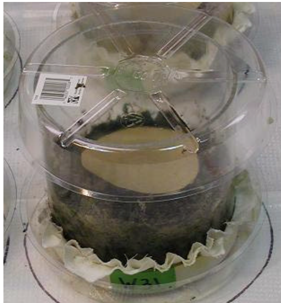
Figure 8-2. Photo of the animal uptake bioassay setup
