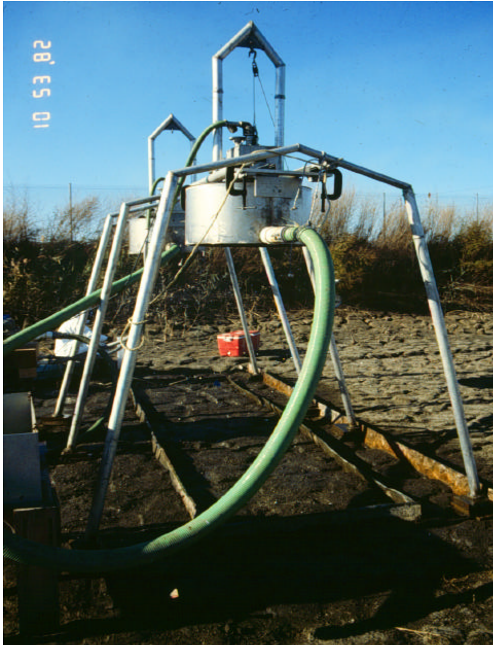
Figure 5-4. Photo of the Rainfall Simulator/Lysimeter System (RSLs)
