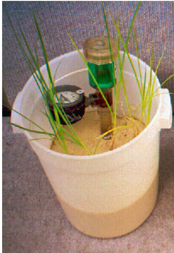
Figure 9-2. Photo of the plant bioassay test setup
