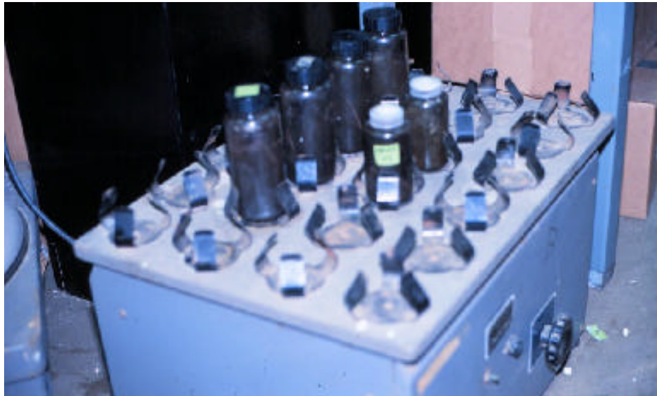
Figure 6-4. Photo of Sequential Batch Leachate Test setup
