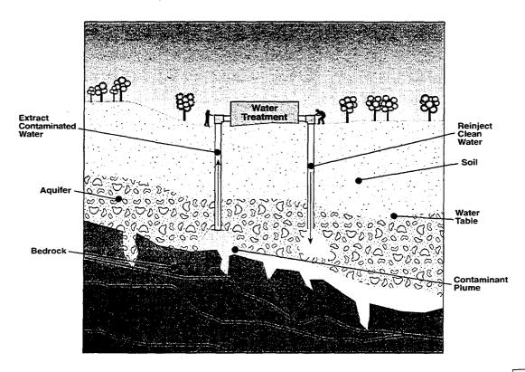
Pumping and Treating Contaminated Ground Water
