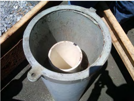
1340 – PHOTO – 300 – View of PW-24A – West toward railroad tracks and Second Lake – good steel casing present, locked well, measurement point present
