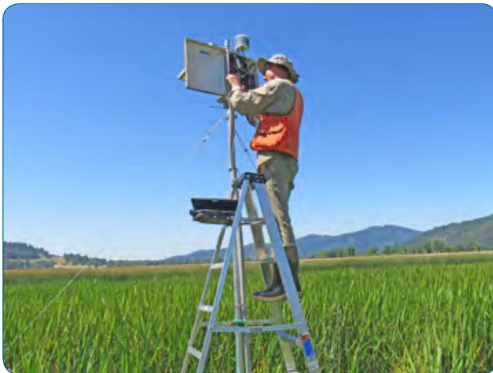
EPA's Office of Research and Development recently installed two data stations in Lane Marsh, in the lower Coeur d'Alene River Basin. The stations are collecting important environmental data to inform research on in-place methods to clean up lead in marsh sediments.
