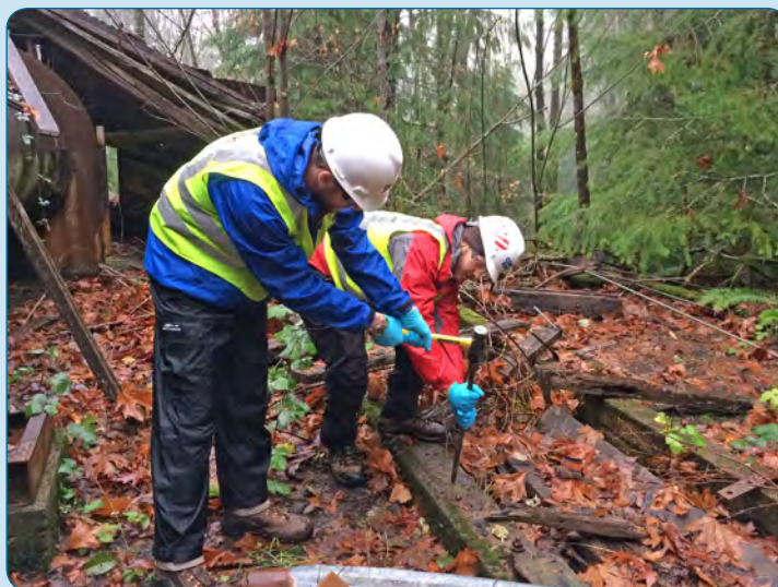
Sampling building materials from one of the former furnace areas. Figure 5 –
