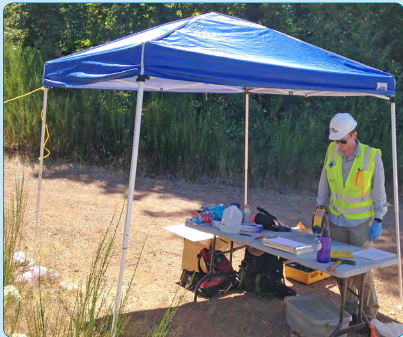
Figure 4 – Field screening soil for metals using an X-ray fluorescence (XRF) analyzer.
