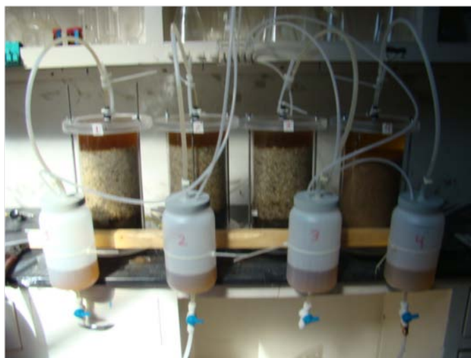
Exhibit 2-7. Completed and operational column test setup.
