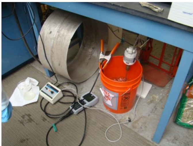
Exhibit 2-3. Large batch neutralization pre-treatment test setup.
