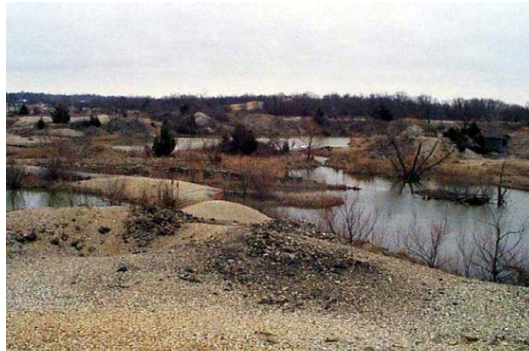
Subsidence pits and chat piles formerly covered the site. Source: Missouri Department of Natural Resources
