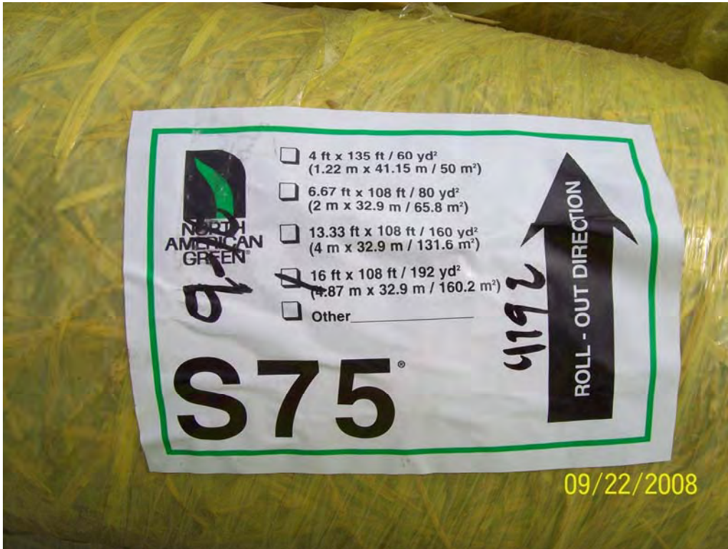
Photograph No. 21 _____ September 22, 2008 Photographer: Chris R. Goffard Signature: Chris R. Goffard Erosion control matting utilized on Area 1 and Area 2 Final Cover.
