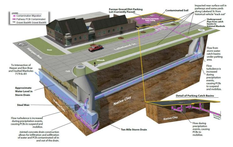
These illustrations show the various routes the PCB contamination took to infiltrate the Ten-Mile Drain Superfund site. Investigators believe it all started many years ago when PCB-contaminated oil was dumped or used for dust control on a formerly unpaved parking lot seen in the top right-hand corner of the first illustration.
