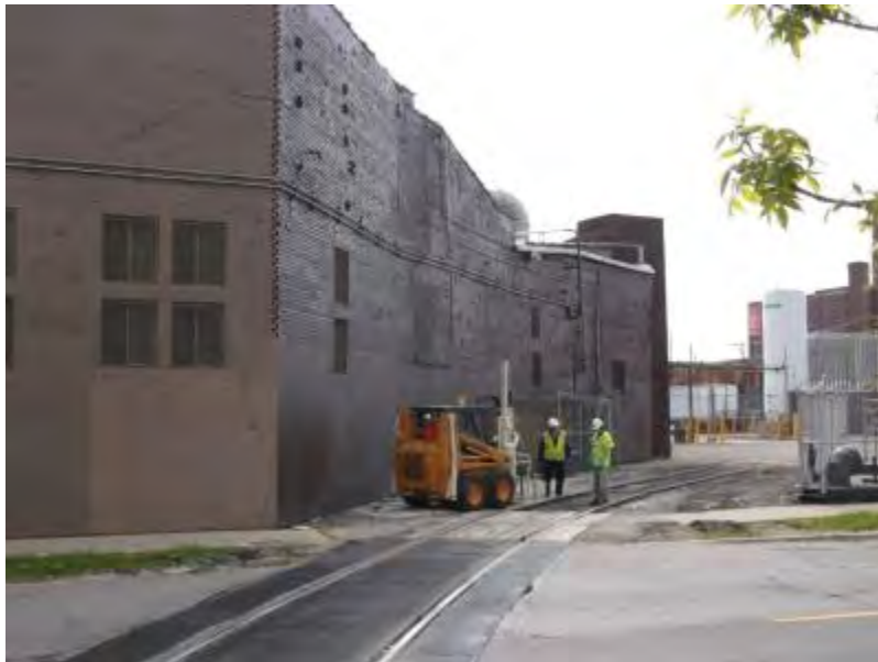
Site: Pilsen Area Soil Site: Railroad/Alley Photo Number: 6 Direction: East Subject: EPA FIELDS advancing Geoprobe at RR-04, adjacent to H. Kramer facility.
