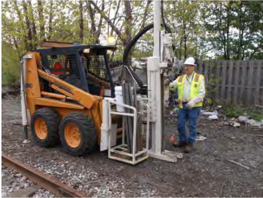
Site: Pilsen Area Soil Site: Railroad/Alley Photo Number: 5 Direction: South Subject: EPA FIELDS advancing Geoprobe at RR-01.
