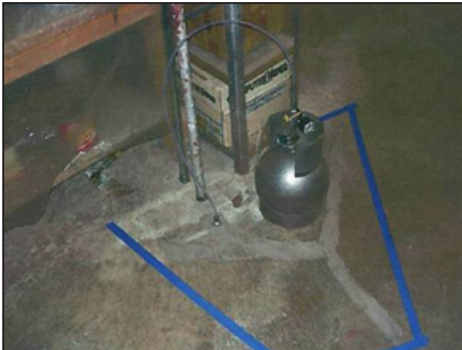
Sub-slab sampling canister and probe.
