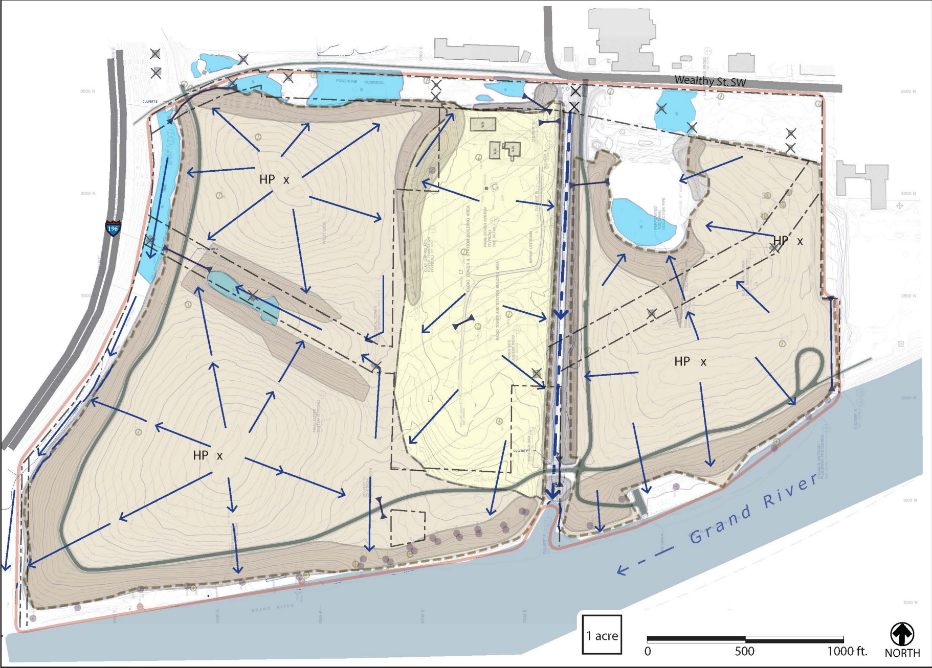
FIGURE 4: SITE STORMWATER MANAGEMENT AND DRAINAGE CHARACTERIZATION
