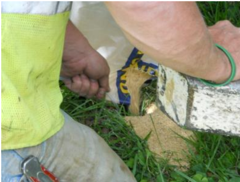
Site: Tuchman Cleaners Site Photograph No.: 16 Direction: Down Subject: Setting of soil gas probe in boring
