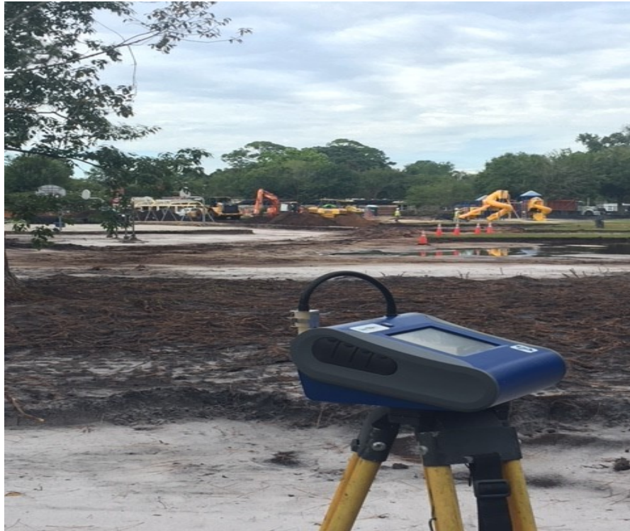
Dust meters to monitoring dust levels
