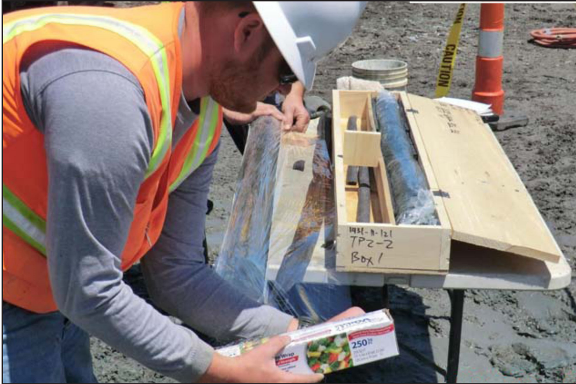
34A – PWS: S&ME logging cores of cured grout for quality control of wall uniformity. May 5, 2011.
