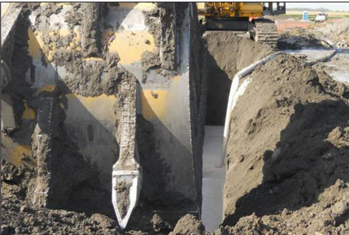
25B – PWS: Rock excavating teeth on bucket of long-reach excavators. April 14, 2011.
