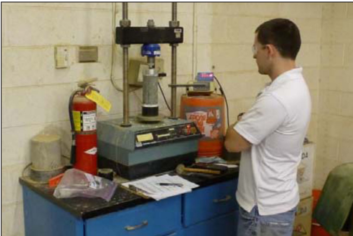
34B – PWS: S&ME laboratory testing sample break for quality control of wall strength. May 2011.
