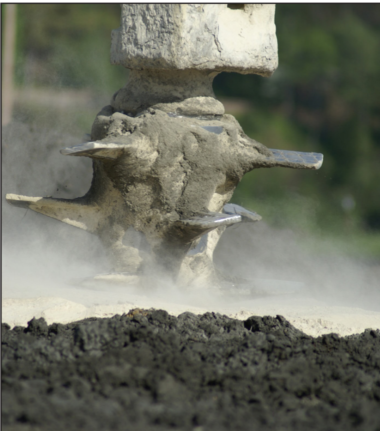
17B – Ash Processing: Using lime treatment; lime mixing equipment. April 13, 2011.
