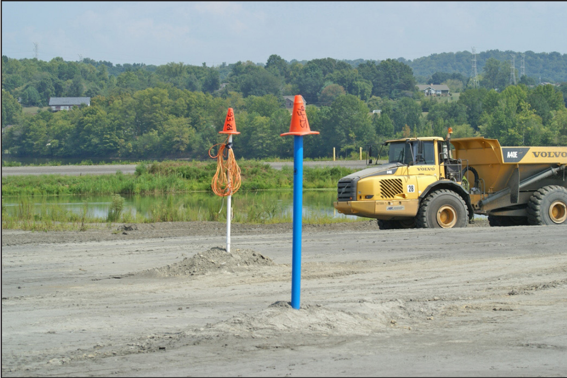
23A – Ash Stacking: Geotechnical instrumentation used for monitoring ash stacking; piezometers (white) and slope inclinometers (blue). August 30, 2011.
