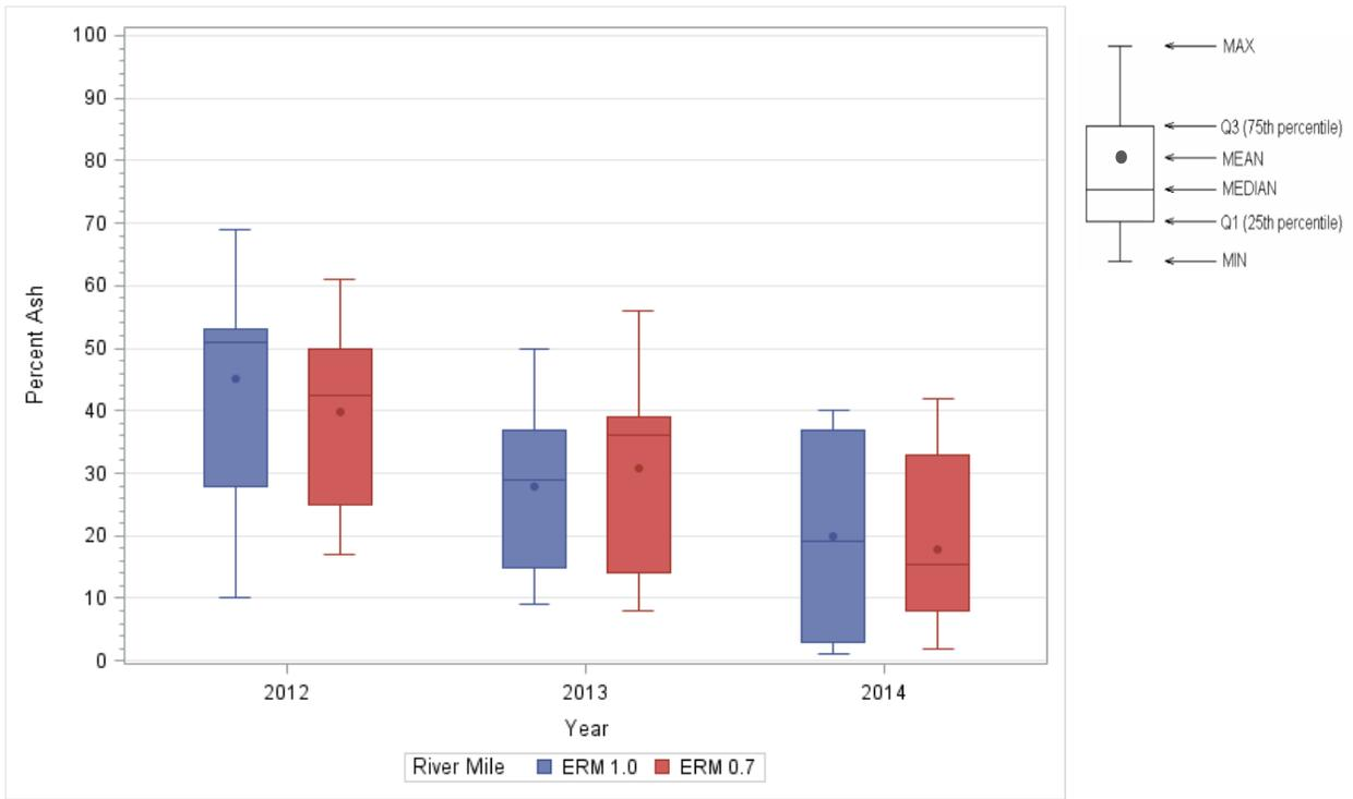
Figure 7. Percentage ash composition in sediment samples collected co-located with benthic invertebrate community samples at ERM 1.0 and ERM 0.7, 2012-2014.
