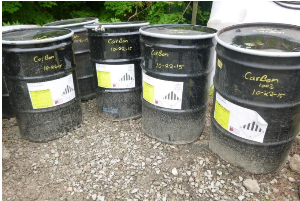
Drums of spent carbon from the aqueous phase treatment system
