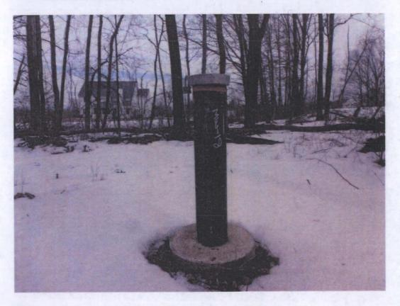
One of three new monitoring wells, MW-18, installed after newest extraction well
