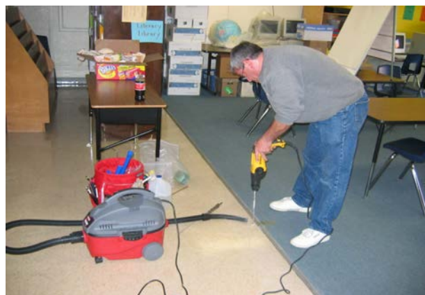
Installing probe for vapor intrusion testing
