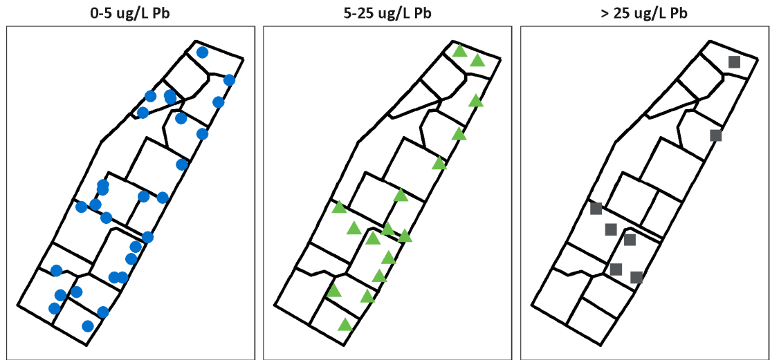
Figure 3: Monitoring Well Locations Grouped by Groundwater Lead Concentrations. These three maps show groundwater monitoring wells grouped by those that have had any lead measurements less than 5 µg/L, those that have had lead measurements between 5 and 25 µg/L, and those that have had any lead measurements over 25 µg/L, respectively. Low groundwater lead levels (<5 µg/L) are widespread at the Site. Lead concentrations are not consistently elevated at the Site; instead, in many wells, exceedances of the groundwater PRG have been transient. Moderate lead concentrations (5 to 25 µg/L) have been detected in wells throughout the Site during at least one sampling period, which suggests the presence of a consistent source of lead, such as would be found in historic fill. The highest concentrations have been found in limited locations across the entire Site and typically during just one sampling period. Only Well MW-107 has had measured lead concentrations higher than 25 µg/L in more than one sampling period.
