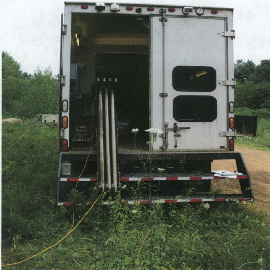
Truck housing for the EC Probe computer and other field equipment.
