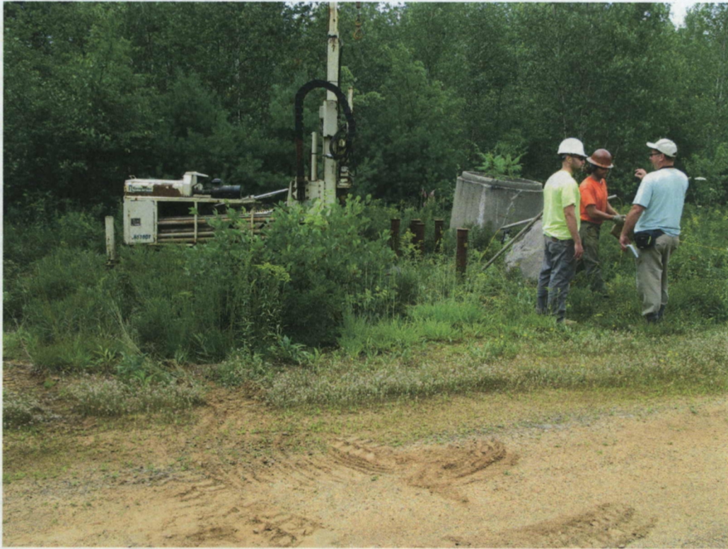
EC Probing at CTW-20 Transect using a track mounted Geoprobe unit.
